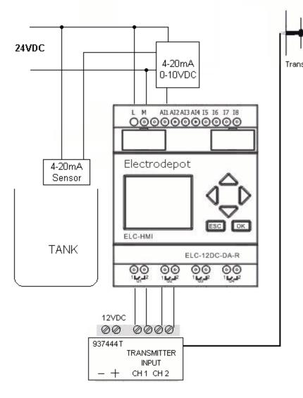
12 VDC and 24VDC Operating Voltage:
