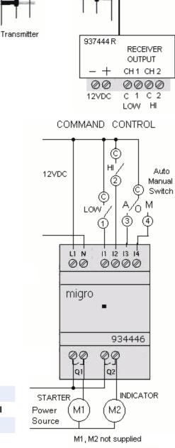
Q1 & Q2 Outputs 5 AMP Class 2 Pilot Duty
